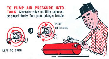
(3) two complete turns to the left. Place thumb over the small hole in handle and pump 35 to 50 full strokes of air into the tank. Then turn pump plunger handle to the right and tighten firmly.
