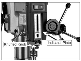
Figure 26. Setting depth stop.
