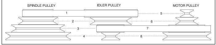
Figure 30. Spindle speed chart.
