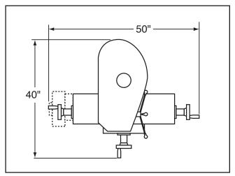
Figure 6. Minimum working clearances.
