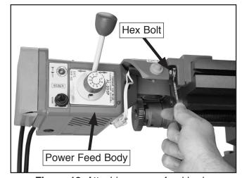
Figure 12. Attaching power feed body.
