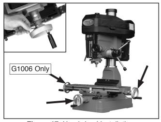
Figure 17. Handwheel installation.
