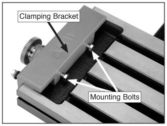
Figure 11. Clamping bracket assembly.
