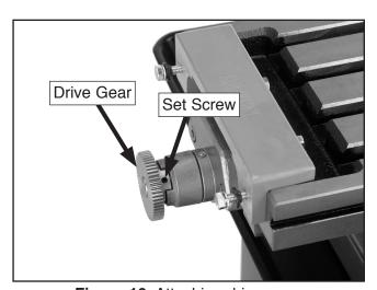
Figure 10. Attaching drive gear.
