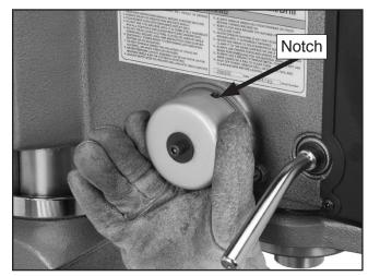
Figure 40. Adjusting spring tension.
