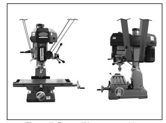
**Figure 7.** Proper lifting strap position.
