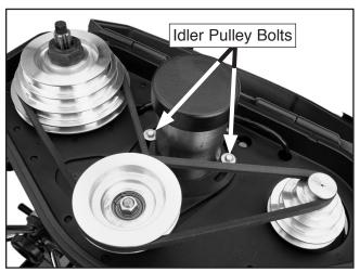
Figure 29. Pulley system.
