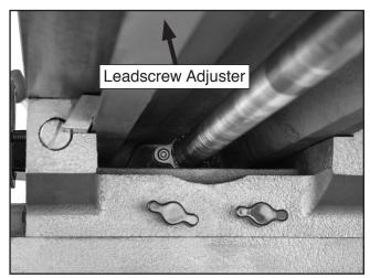
Figure 41. X-plane leadscrew adjuster.
