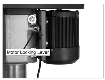
Figure 28. Motor locking lever.
