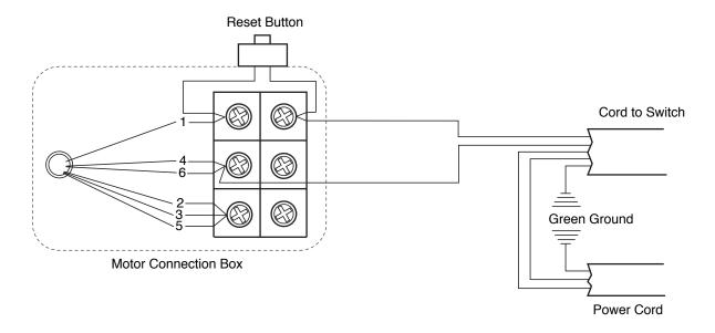
NOTE: For clockwise rotation (facing the end of the shaft) wire as shown above. For counter clockwise rotation, interchange leads 5 and 6.
