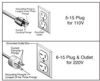
Figure 2. Recommended plug types.
