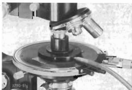
Microscope cooling stage with attached nitrogen chamber and protection tube for screening off air from the outside
