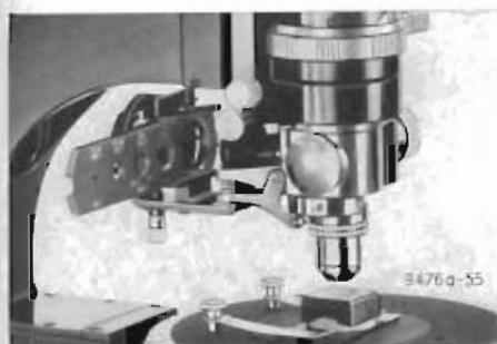
Vertical illuminator for PANPHOT-POL, as above, but with illuminating tube OPORN. Vertical illuminator as supplied for ORTHOLUX-POL and PANPHOT-POL
