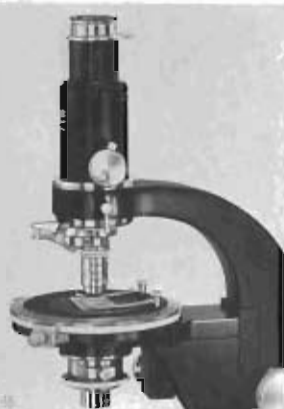
LABORLUX-POL with photographic Pol-tube O 14 and objective centring clutch
