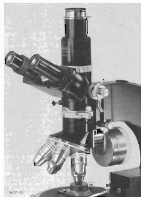
ORTHOLUX-POL with equipment for incident phase contrast illumination
