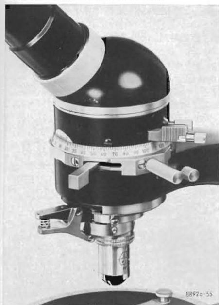
Top of stand with rotating analyser, Bertrand lens system, Pol-tube P 10 with iris diaphragm and objective centring clutch
