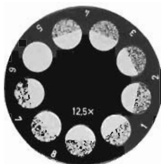
Revolving disc with 8 comparison slides of polished coal specimens and a micrometer plate (for the fusit analysis)
