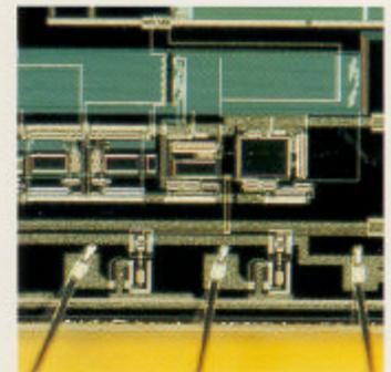
Wire bonding section on the AF sensor
