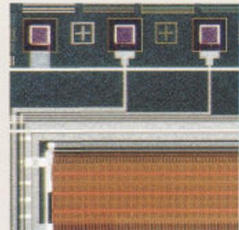
Pattern on the Charge Modulation Device (CMD)
