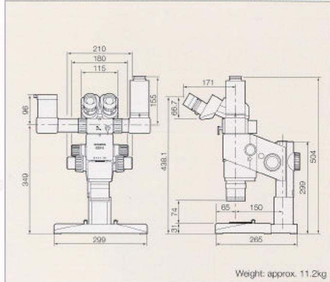
**Photomicrography combination dimensions (SZX-TR30 + 35mm camera back)**
