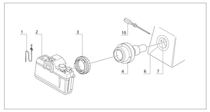
Fig. 2-5 Attachment of 35 mm SLR cameras with camera adapter 2.5× / T2 to front-port of Axiovert 25 C / CFL / CA
