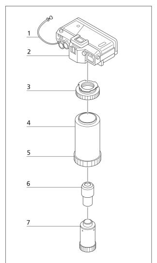
Fig. 2-7 Attachment of 35 mm SLR cameras with objective f' = 63mm to camera port with 40mm clamping diameter
