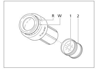
Fig. 2-2 Attachment of photo reticle MC 2.5× in eyepiece
