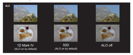
ALO works with both JPEG and RAW images. With RAW images, photographers can choose the same settings that the camera offers when processing the images in the supplied DPP software. You can select from Standard, Low, Strong or Disable. With previous EOS DIGITAL cameras having ALO, the function worked only in the P, Tv, Av and CA modes. However, with the EOS-1D Mark IV, ALO now also works in the Manual mode and bulb as well, in keeping with the idea of enhanced JPEG workflow.
