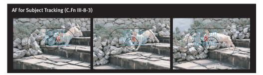
C.Fn III-8-1, III-8-2 or III-8-3 must be on for C.Fn III-4 (AI Servo AF tracking method) to become fully effective. The exception occurs when using Automatic Focusing Point Selection, in which case both settings for C.Fn III-4 are effective even when C.Fn III-8 is off.
